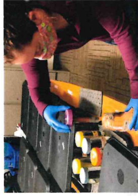
In 2020 and 2021, Water Bureau engineers tested Bull Run water in jars to determine the most effective corrosion treatment to use at the Bull Run filtration facility.
